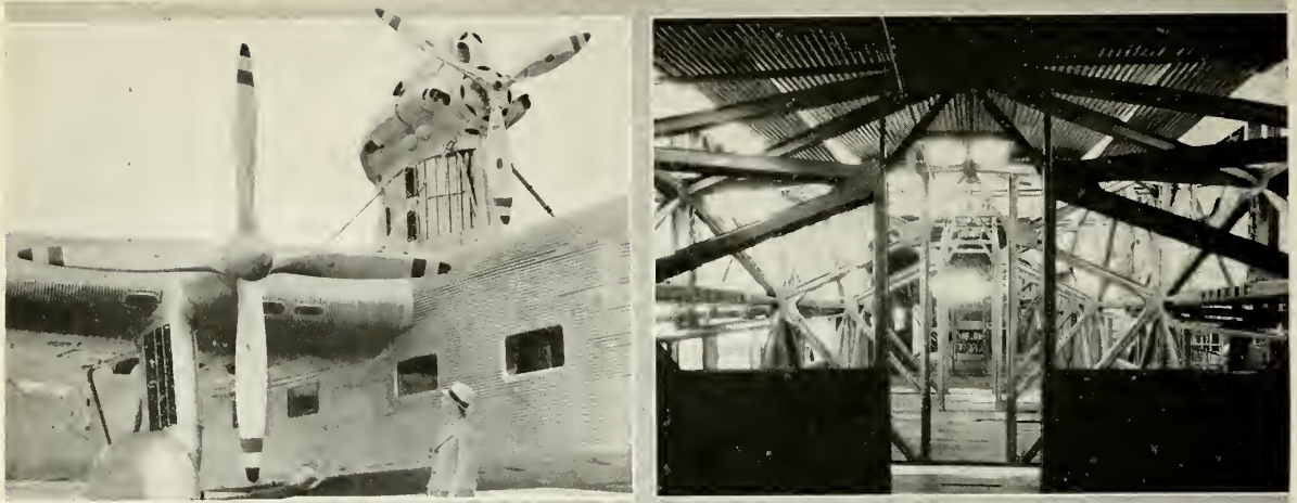
Power plants of the Ford model 14-A and an interior view of the cabin during construction
